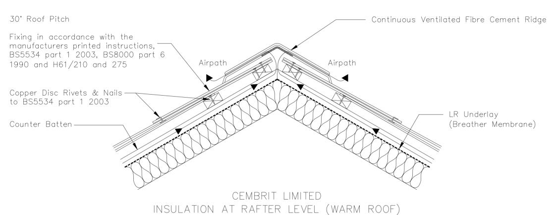
VENTILATED FIBRE CEMENT RIDGE TYPICAL DETAIL
